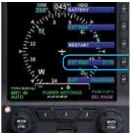
Figure 6-4 External Power Voltage Status
