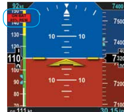
Figure 6-3 Battery Charge Remaining
