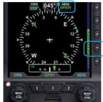
Figure 6-9 Operating in GPSS Mode
