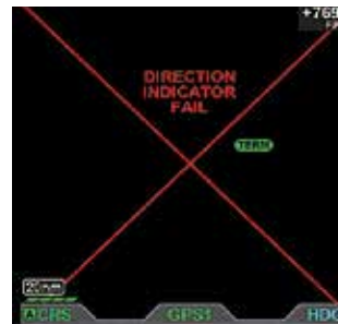
Figure 4-51 Direction Indicator Fail
