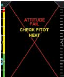
Figure 4-9 Pitot Obstruction with Failed GPS
